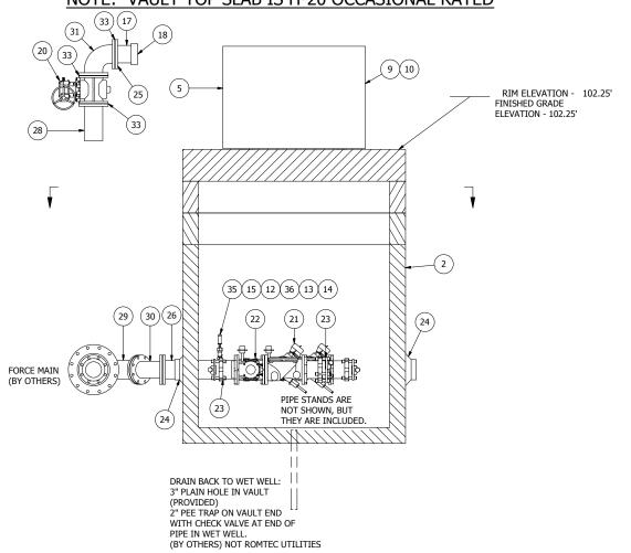
6' X 8' VALVE VAULT **6" PIPING AND VALVES** 12" PUMPING PORT
