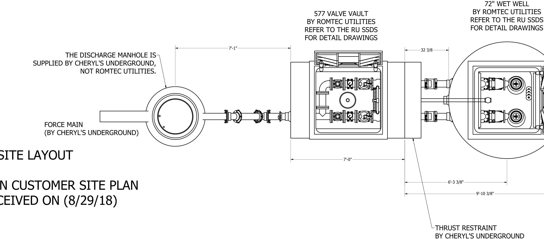
CARB SAMPLE SITE LAYOUT 9/4/18 BASED ON CUSTOMER SITE PLAN DWG RECEIVED ON (8/29/18)
