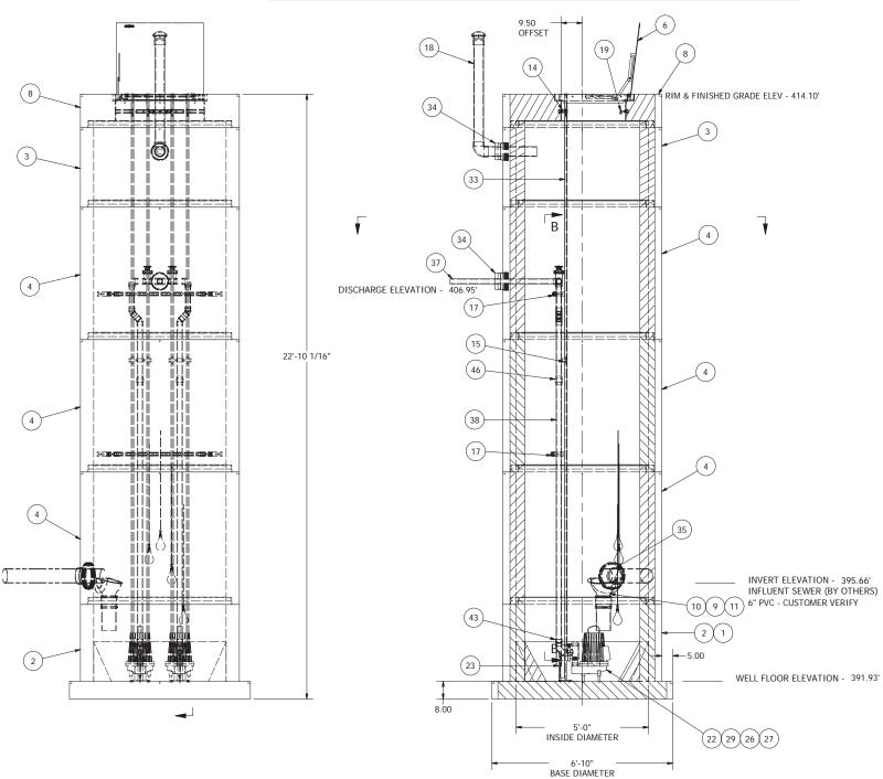
NOTE: ALL DIMENSIONS AND ELEVATIONS SHOWN ARE NOMINAL DIMENSIONS. IT IS THE RESPONSIBILITY OF THE ON-SITE CONTRACTOR OR ROMTEC UTILITIES CUSTOMER (NOT ROMTEC UTILITIES) TO VERIFY THE ACCURACY OF ANY CRITICAL DIMENSIONS OR ELEVATIONS PRIOR TO SETTING OR INSTALLING ANY EQUIPMENT.
