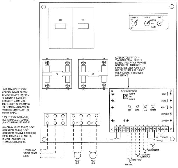
**NOTE**: Panel is not to be used with pumps that do not include capacitors.
