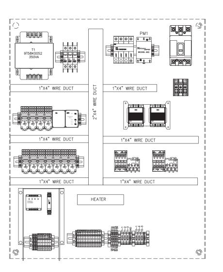
THE ENCLOSURE SHOWN REPRESENTS THE INTENT OF THE DESIGN. OFTEN THE ENCLOSURE SIZE AND LAYOUT MUST CHANGE TO ACCOMMODATE THE REQUIRED COMPONENTS AND FINAL DESIGN. PLEASE CONTACT ROMTEC UTILITIES TO OBTAIN ACTUAL AS-BUILT DRAWINGS BEFORE INSTALLATION.
