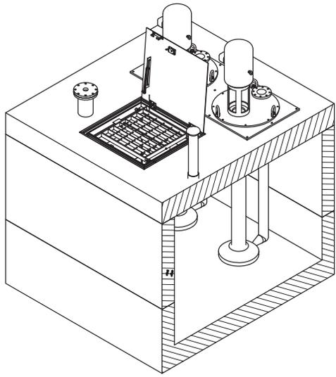
FLOAT, PRESSURE TRANSDUCER AND TEMPERATURE MONITOR CABLES ARE TO BE ROUTED UP THROUGH THIS SPOOL AND 2in TAPPED HOLE.
