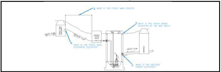
Source of Water: **Power Plant** Water Type: Process Water - Hot Water (120 degrees max) Peak design inflow (max flow to lift station): 850 g.p.m. @ 25 ft. TDH 850 g.p.m.
