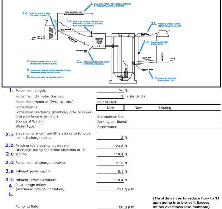
None Permanent Portable None Don't Know **6.** Standby generator requirement: Diesel Natural Gas Propane Standby generator fuel: 208V 208V 240V 480V 7. Available power supply: 3-phase Single-phase 3-phase Yes Yes <u>No</u> Is this lift station considered a classified space?
