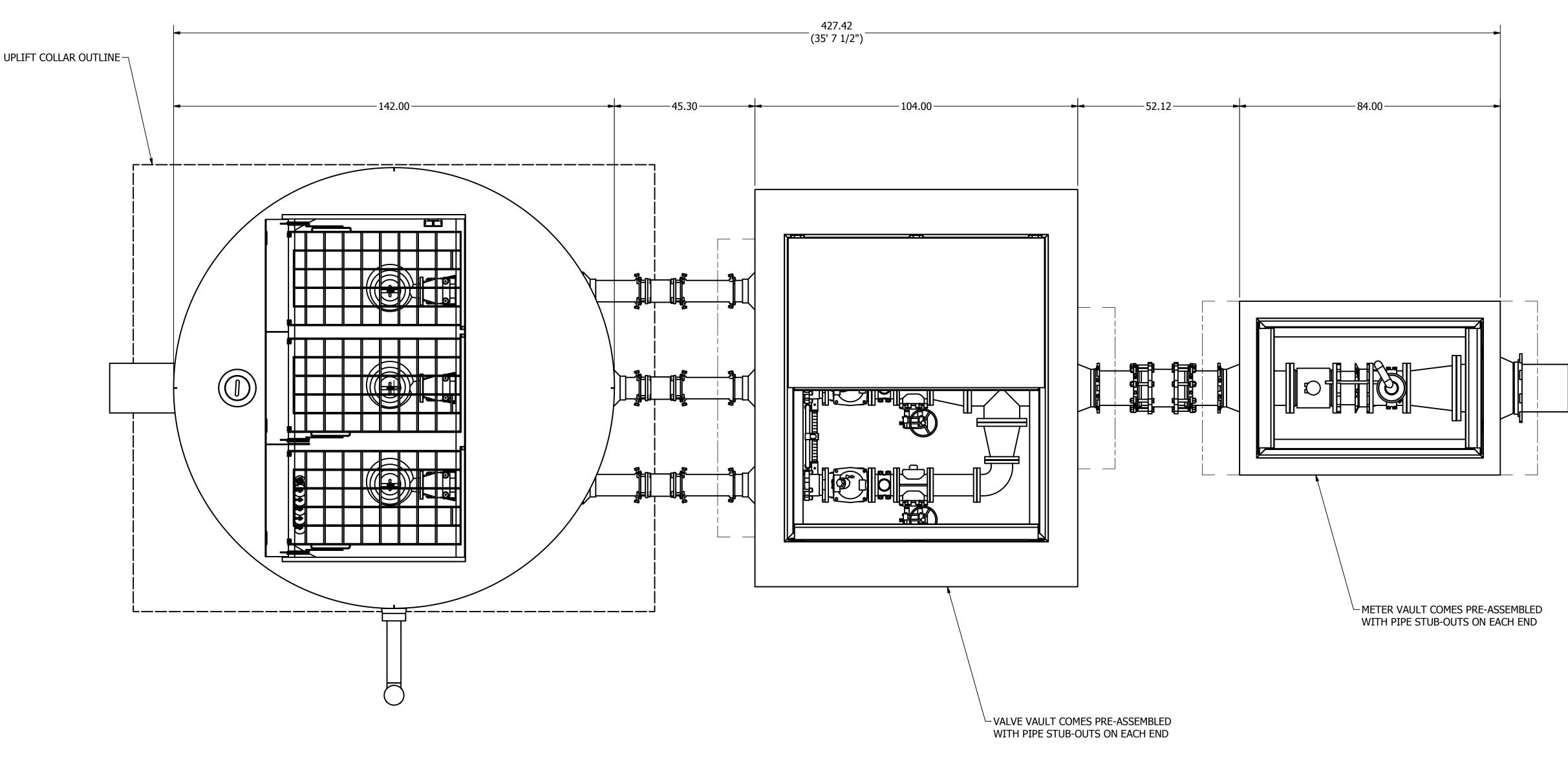
NOTE: ROMTEC UTILITIES IS PROVIDING ALL PIPING AND FITTINGS AS SHOWN. ALTERING THE DISTANCE BETWEEN THE WELL AND VAULTS WOULD REQUIRE ADDITIONAL PIPING AND FITTINGS (PROVIDED BY OTHERS AS REQUIRED)
