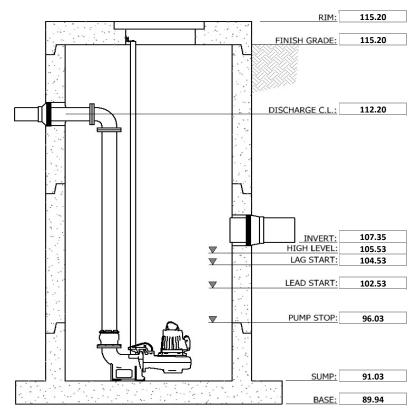
Note: Image is a preliminary representation of the pumping system. Elevations shown are the primary factors used for sizing the wet well. Backup levels not shown. Additional (or fewer) level settings may be required.
