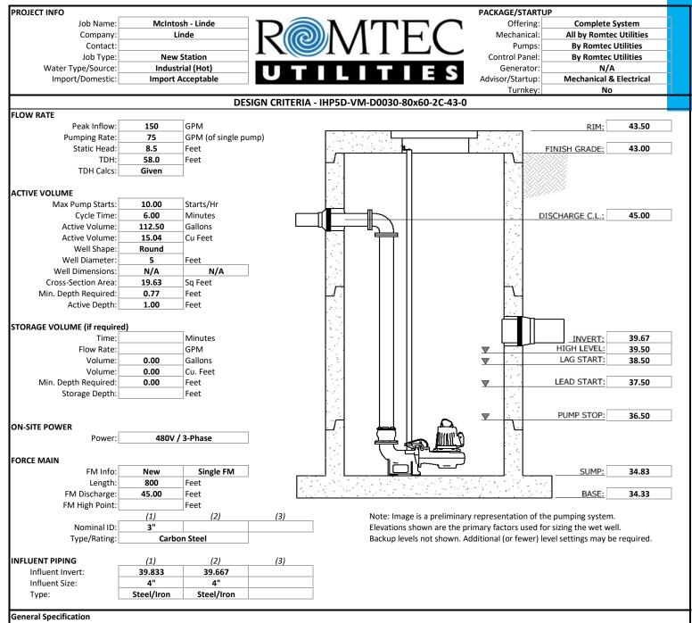
A. The package pump station supplier of the sewer lift station shall be Romtec Utilities. The package pump station supplier shall design and draw the complete lift station including the wet well structure and associated piping and valves along with the control panel and the associated schematics.
